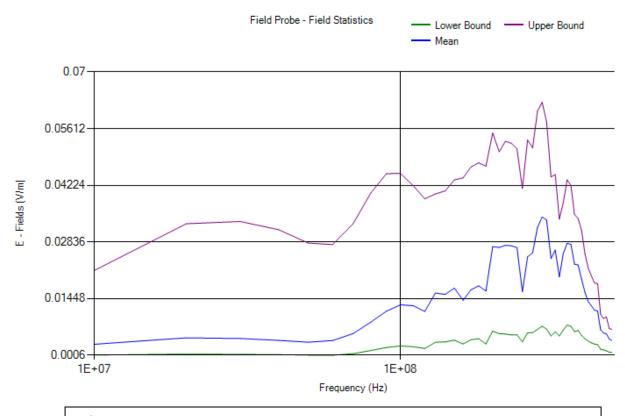
**NOTE**: Frequencies outside the range of frequencies specified in the domain section should be interpreted with extreme caution, as the time and spatial steps were not calculated to properly capture frequencies outside of those specified.
